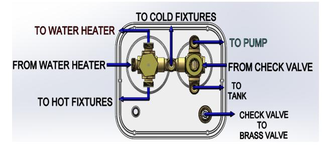
DRY CAMPING - TO RUN HOT AND COLD FIXTURE FROM STORAGE TANK (VIA RV PUMP)
