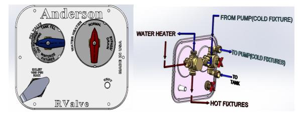
**CITY FIXTURES-**TO RUN FIXTURES FROM PRESSURIZED CITY WATER
